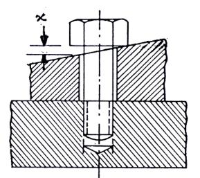
4.4.1.1.2F- Development of bending stress in a bolt
