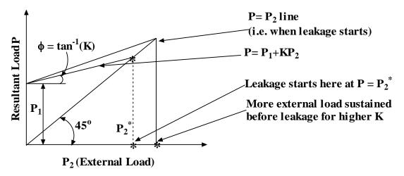
4.4.3.1F – Force diagram for joint separation
